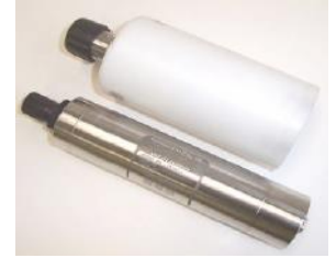
2 x Pressure sensors (7000 m full scale) (1mm accuracy)
